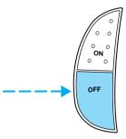
Once speed control is switched off, the previously programmed set speed will be erased.
